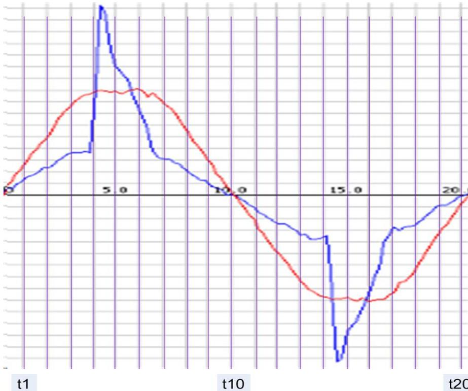
Sample rate of approx 1024 samples per second equates to approx one measurement every millisecond and only 20 measurements per cycle at 50hz. At 800Hz it equates to 1.25 measurements per cycle. In the example waveform the Peak current would be missed.
