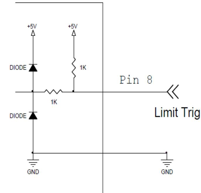
Figure A-1 Connection of Limit Trigger
