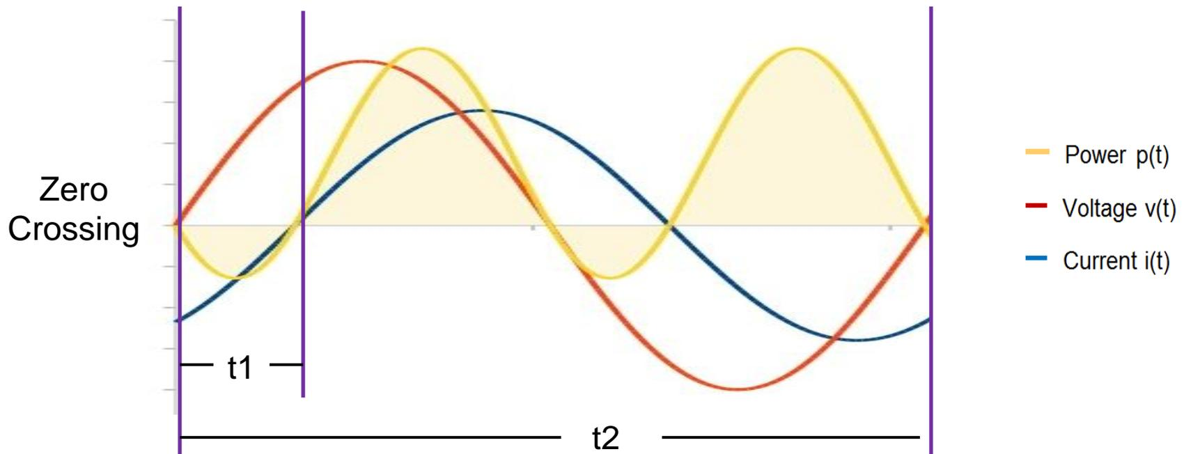
Power Factor = the Cosine of the Phase angle of the current versus voltage waveforms.
