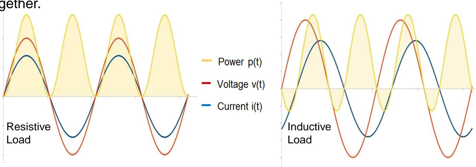
True Power or Watts =  $V_{rms} \times I_{rms} \times \cos \theta$
